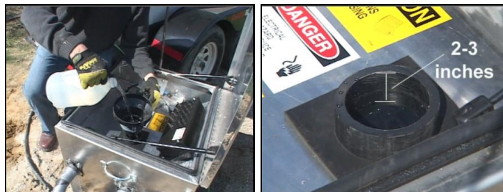
Figure 16. Fill the Standing Column for a 2-3 in/ 50-75 cm Air Gap at the Top
