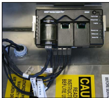
Figures 7A. Attaching Sensor Leads to the Data Logger
