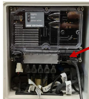
Figures 7A. Attaching Sensor Leads to the Data Logger
