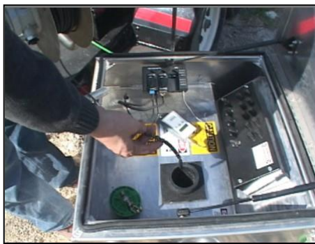
Figure 10. Inserting the Temperature Probe into the Standing Column
